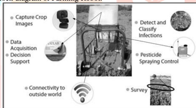
FIG.2. SCHEMATIC DIAGRAM OF FARMING ROBOT [2].
