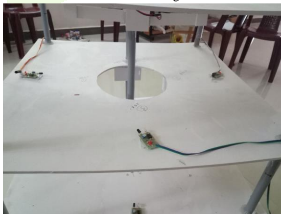
Figure:8 shows the IR sensor arrangement in each slot.
