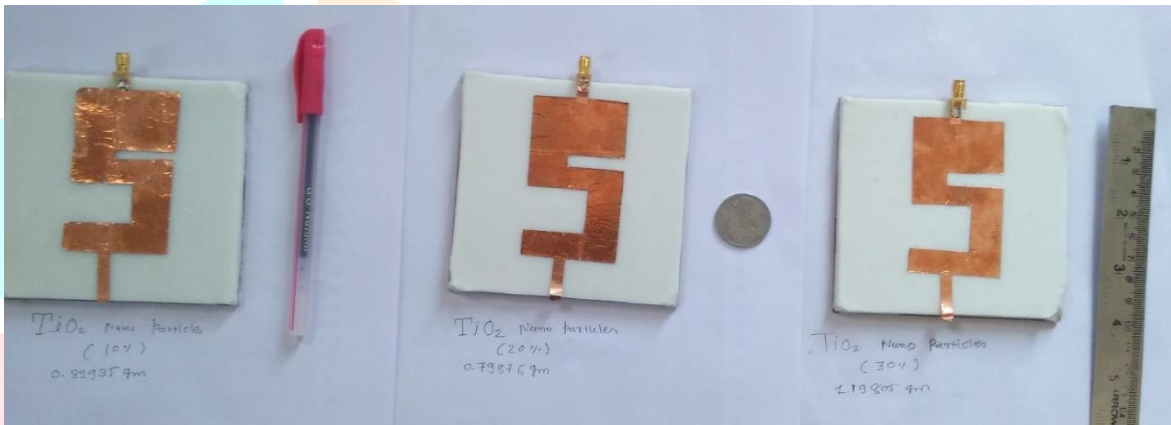
Fig.7 Fabricated S shaped model with 10%, 20% and 30% TiO 2 Nano particle
