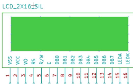
Fig1.7 Pin diagram of LCD
