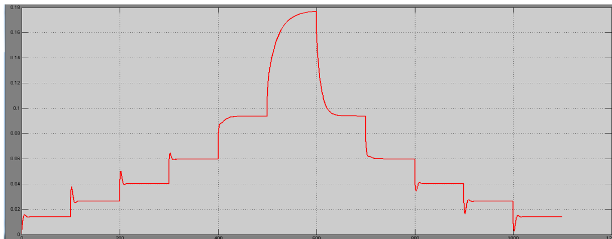
Fig. 1-9: Throttle Variation during Staircase Response
