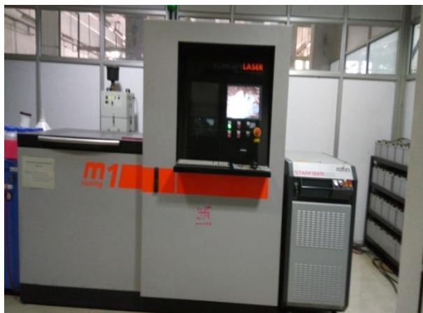
Figure 1 Experimental Set up Concept Laser M1
