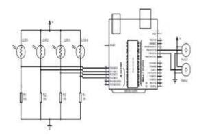
LDRs are used as the main light sensors. Two servo motors are fixed to the structure that holds the solar panel. The program for Arduino is uploaded to the microcontroller. The working of the project is as follows.
