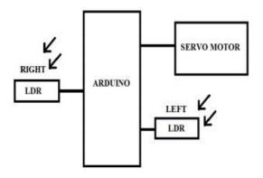
The circuit design of solar tracker is simple but setting up the system must be done carefully.
