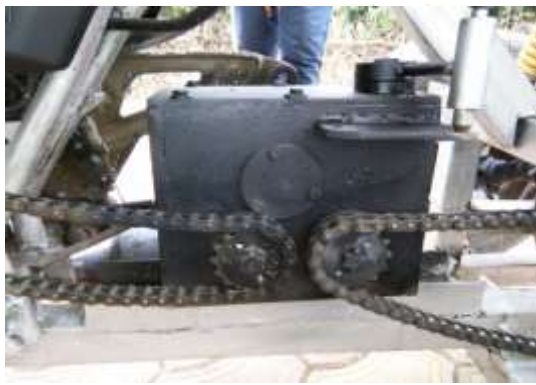
Fig. 2: Reverse gearbox installed in quad bike.
