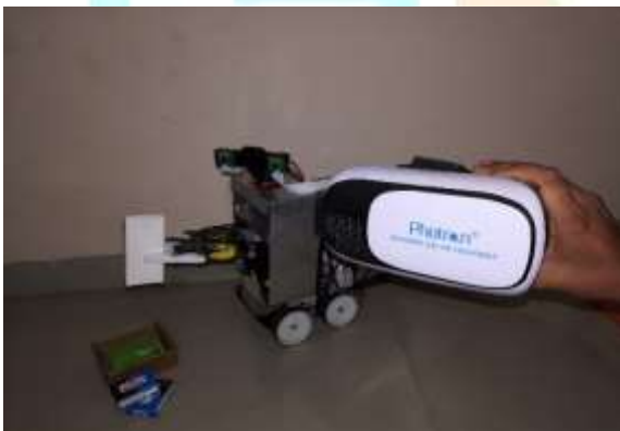
Fig 3: VR headset's left and right orientation followed by camera on robot.
