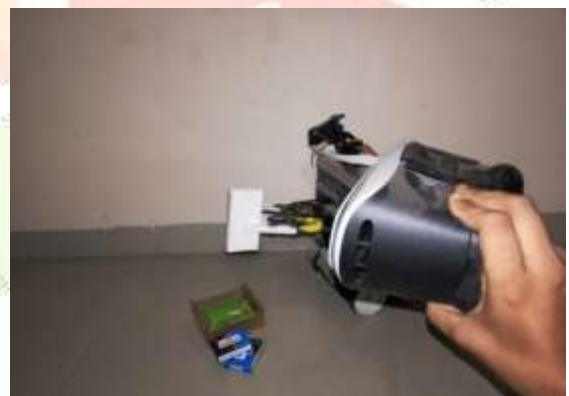
Fig 2: VR headset's upward and downwards orientation followed by camera on robot.
