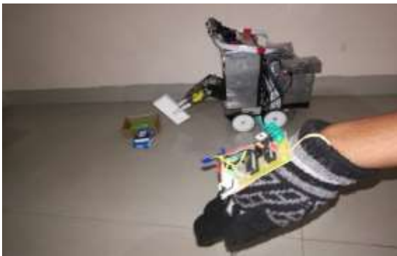
Fig 1: Hand gesture for controlling picking object & lifting up operation.
