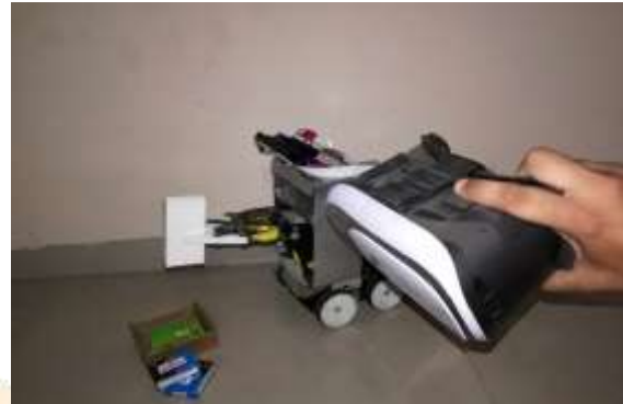
Fig 2: VR headset's upward and downwards orientation followed by camera on robot.
