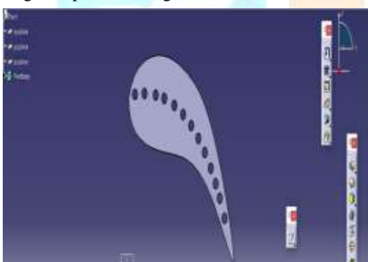
Fig: Modeling of a turbine blade with 13 cooling holes
