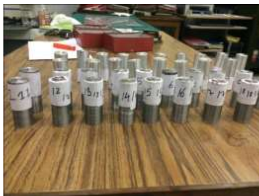
Fig . Mild Steel (EN8) round bars.
