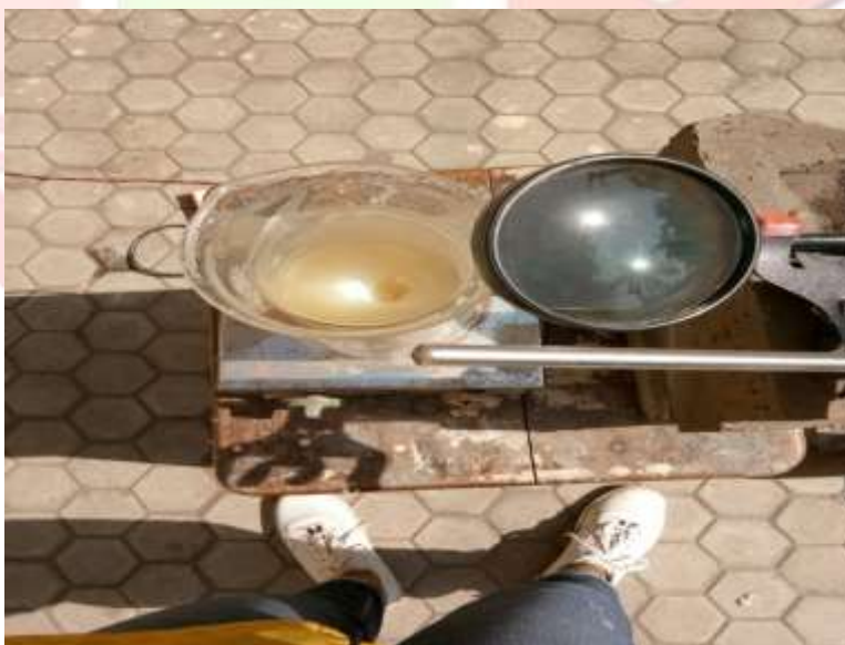
Figure 2: Solar Photo Fenton Reactor
