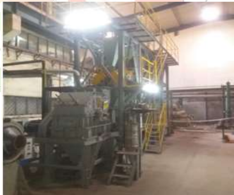
Figure 7 Pilot Scale Pot grate sintering machine
