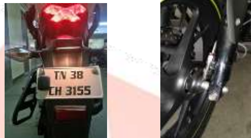
Fig.8 & 9 GPS antenna and Proximity sensor fixed to bike
