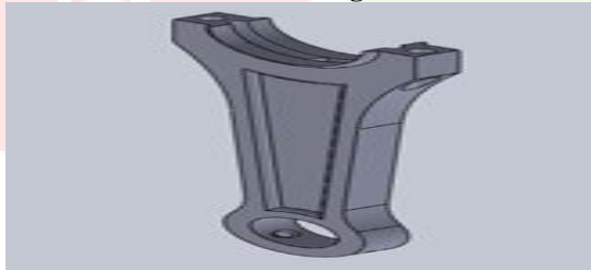
3d modeling of a connecting rod
