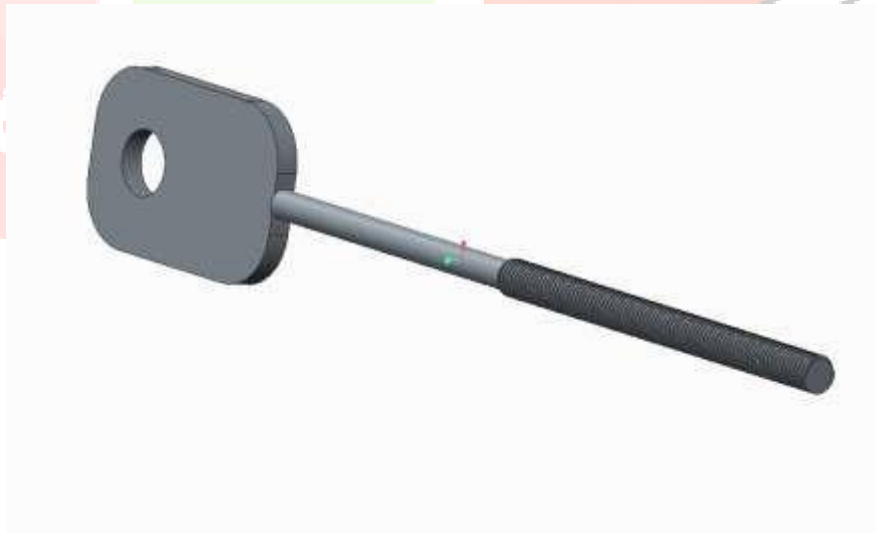
Figure 21: The shaft limb which provides assisting torque to the leg
