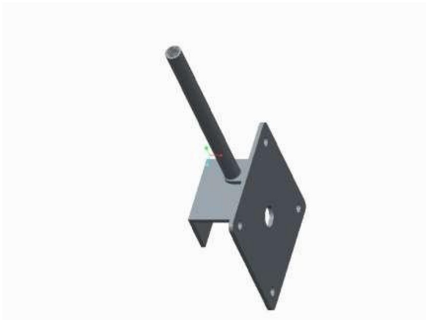
Figure 22: The lower limb which provides length adjustment and motor mount
