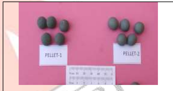
Fig. 1: Prepared pellets from Daitari iron ore ultra-fines.
