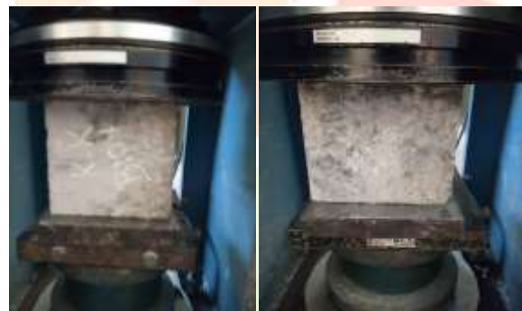
Fig.2: Testing of Cubes in Compression Testing Machine
