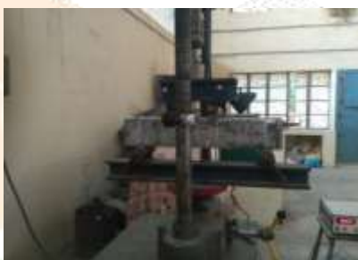
Fig.4: Flexure Strength Testing of Prism
