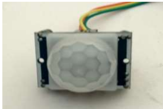
Figure 4. Actual View of PIR Motion Sensor
