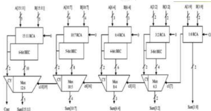
Fig (ii). Modified carry select adder
