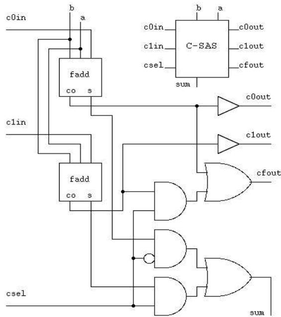
Fig [2] arithmetic operation of CSA Adder
