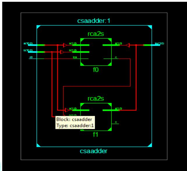
Fig (iii). CSA Adder Schematic view
