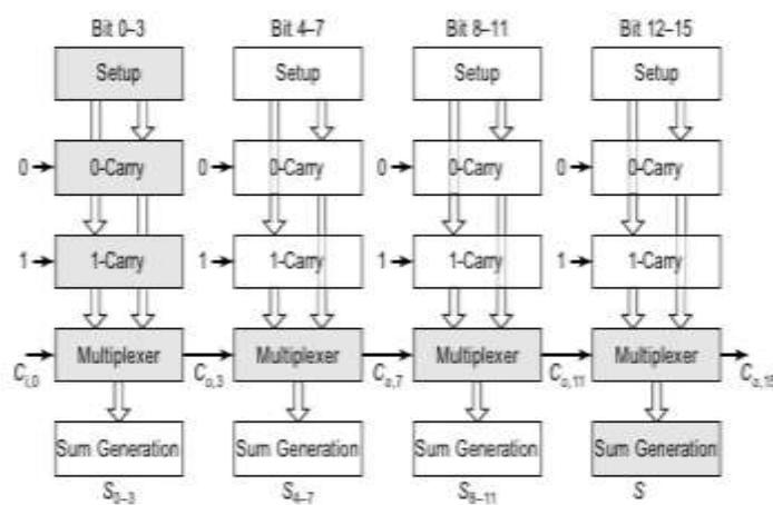
Fig [7] Critical path for CSA Adder
