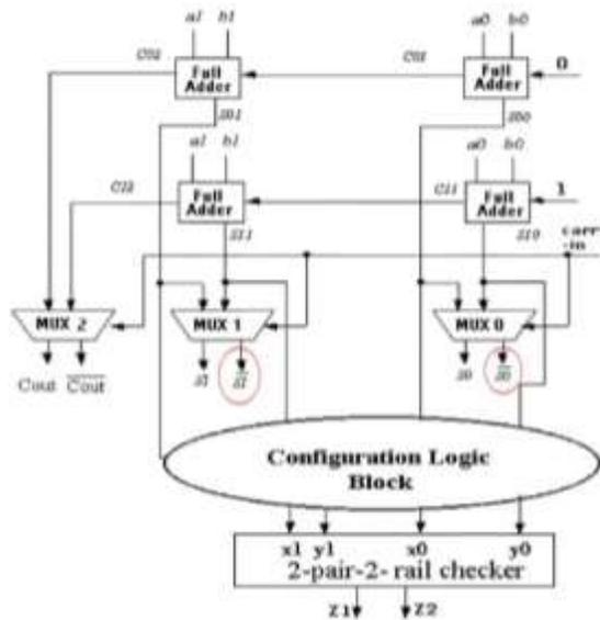
Fig [3]. 2-bit carry-select Adder
