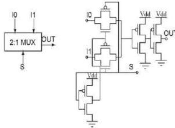
Fig [5] basic circuit diagram for MUX
