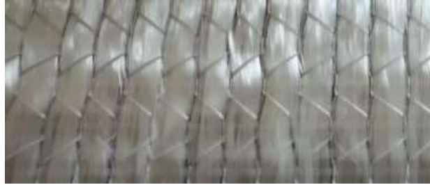
Fig 1. Unidirectional Glass fiber Hybrid Resin
