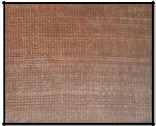
Fig. 4 Manufactured specimen of Glass fiber reinforced Epoxy composite with 5% of Polybenzamidazole
