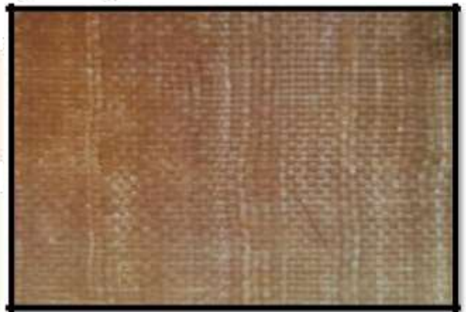
Fig. 5 Manufactured specimen of Glass fiber reinforced Epoxy composite with 10% of Polybenzamidazole
