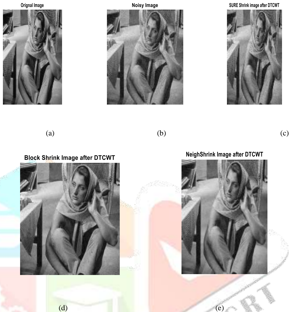
Fig 8: DT-CWT based Denoising on Barbara Image (a) original Barbara Image (b) Barbara Image with Gaussian Noise of variance 10 (c) Denoised Image with sure shrink (d) Denoised Image with Block shrink (e) Denoised Image with Neigh shrink
