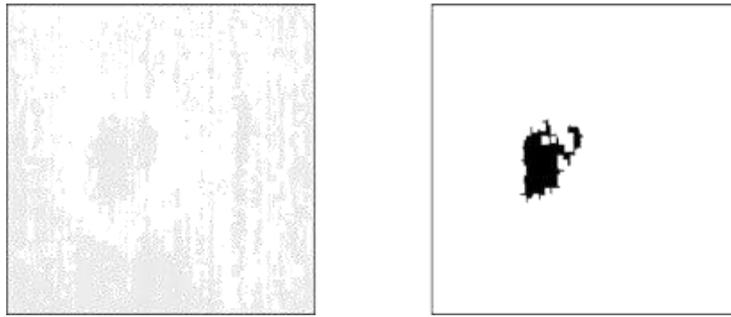
Fig 13: Tiles with large water drop defect
