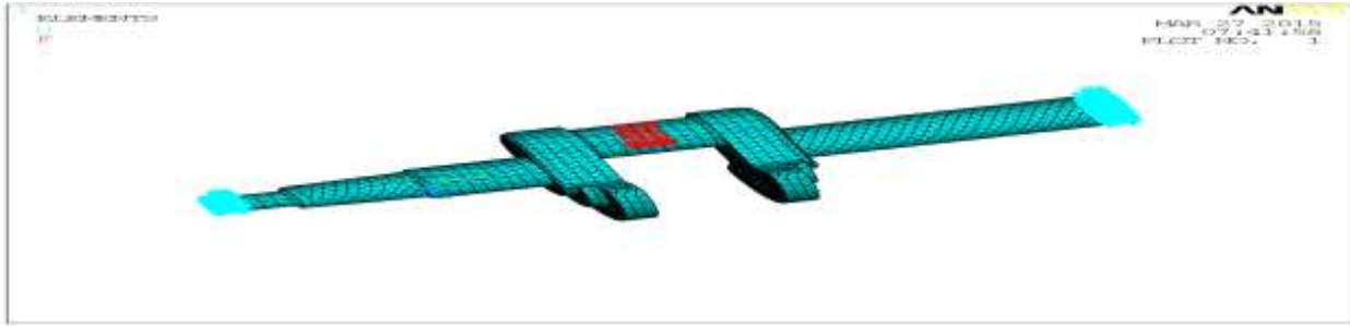
Fig.4 Boundary conditions of Crank shaft
