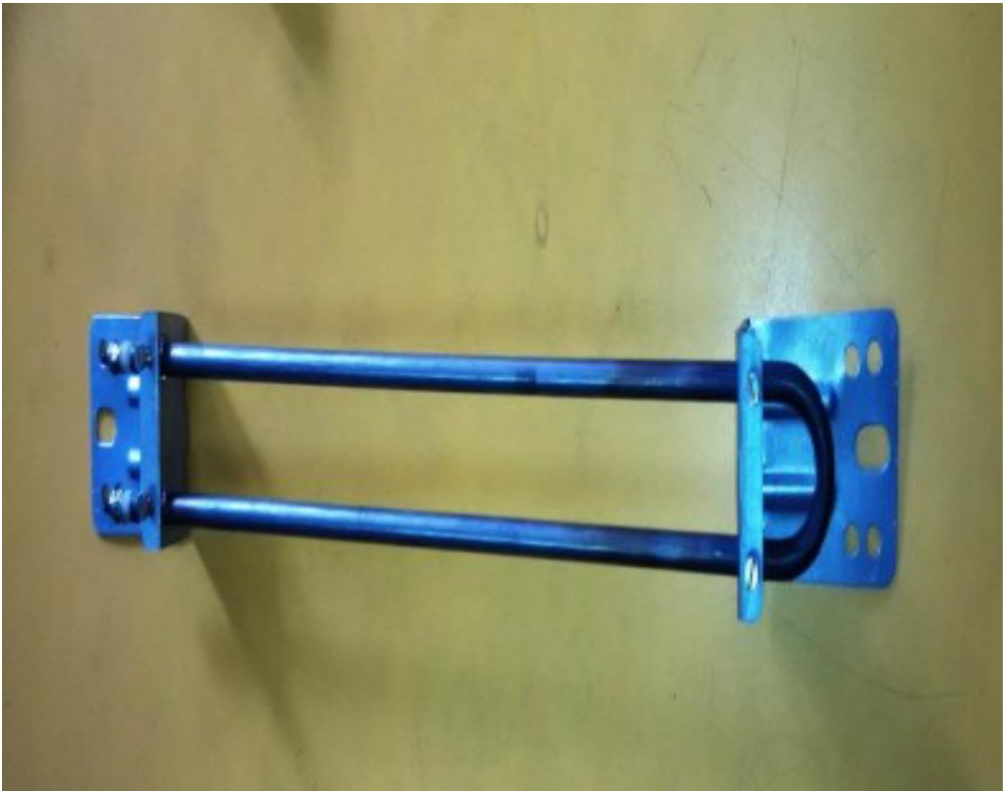
Fig.15: electric heater without fins
