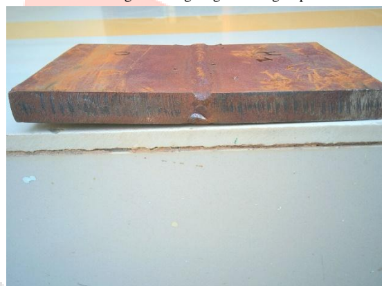
Fig 3. 0-degree groove angle specimen
