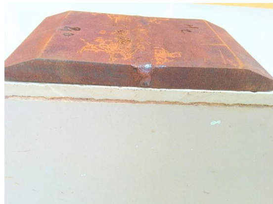
Fig 1. 40-degree groove angle specimen
