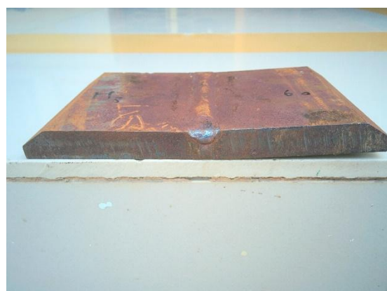
Fig 4. 60-degree groove angle specimen
