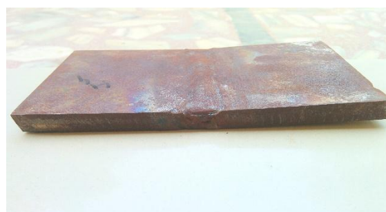
Fig 2. 80-degree groove angle specimen
