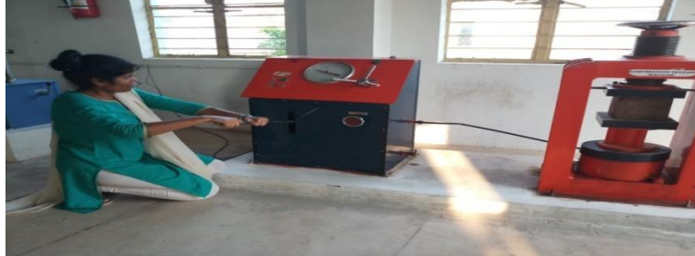
Fig. 3: Compressive strength test
