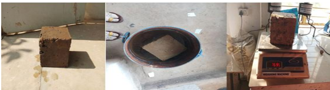
Fig. 2: Water absorption test conducted in lab
