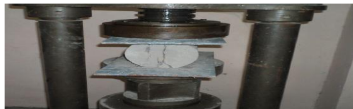
Fig. 5. Split tensile strength test
