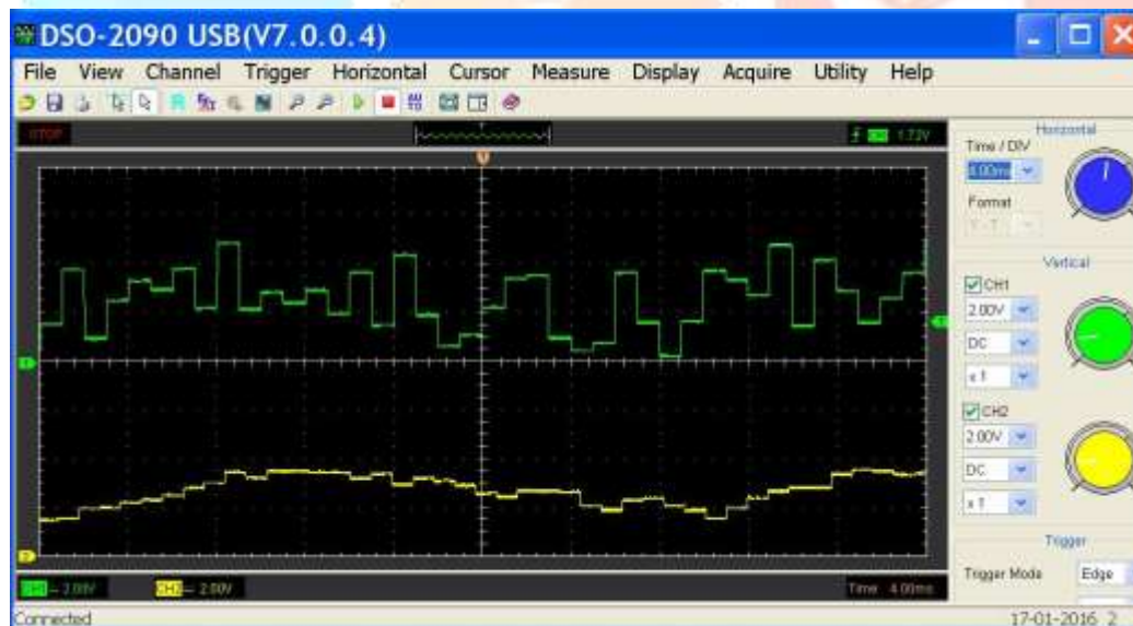
Fig. 5. Oscillogram of signals: CH1 - the filter input signal; CH2- the filter output signal
