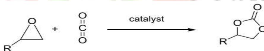
Figure 1.4 Cycloaddition of CO 2 to epoxides to form cyclic carbonates, general reaction. R = alkyl/aryl group
