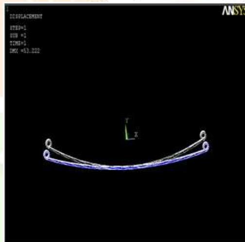
Fig.6: Deflection of Master Leaf (Steel)
