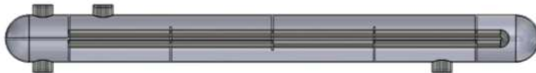
Figure 3 U-Tube type Heat Exchanger _ proposed type
