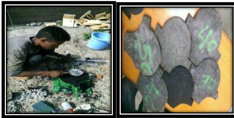
Fig.-7 Sample products of plastic roof tile
