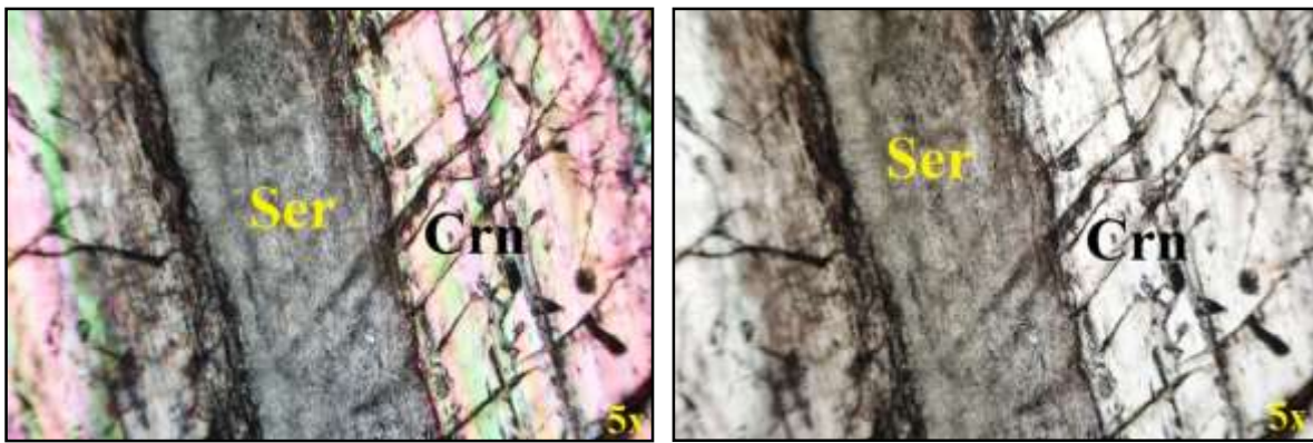
Fig.2. Bigger size Corundum under PPL and XPL
