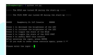
Fig 10: Screenshot showing the Raspberry Pi IoT console
