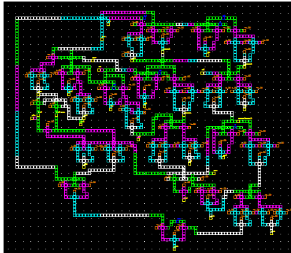
Figure 20. QCA layout for the ALU.
