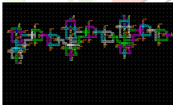
Figure 14. QCA layout for the Ripple carry adder.
