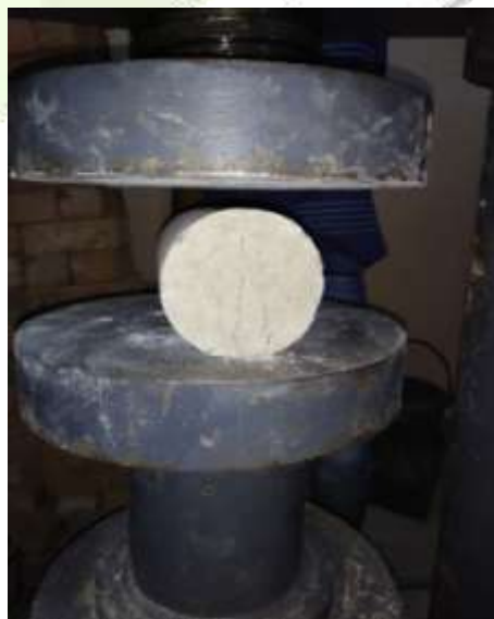
Figure 2.0 Testing cylinder specimens in a CTM
