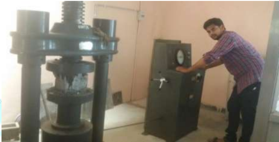
Figure - 1.0 Compressive test on concrete cube.
