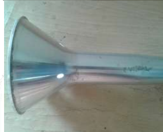
The above figures show surface roughness and scratch on the surface of spike support
