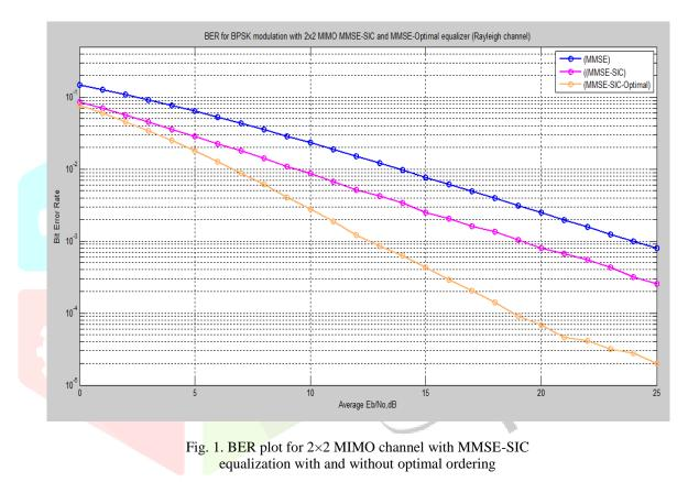
The figure.1 shows the BER performance between MMSE equalization with simple SIC case and SIC with optimal ordering .The figure indicates that at BER of  $10^{-3}$ , the MMSE equalizer shows SNR ~24 dB ,for MMSE-SIC case ~19dB. The MMSE-Optimal case SNR is ~13dB.Between the MMSE-SIC and optimal ordering there is a significant improvement in the SNR ~ 6dB.
