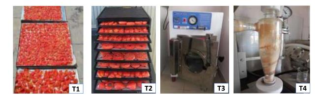
Fig.1 Drying methods and performing of drying processes: T1: Sun drying; T2:Oven drying; T3: Vacuum drying; T4: Spray drying
