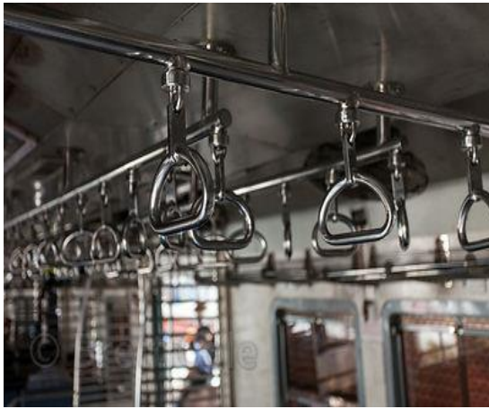
Fig. 01. Overhead grab handle in local train
