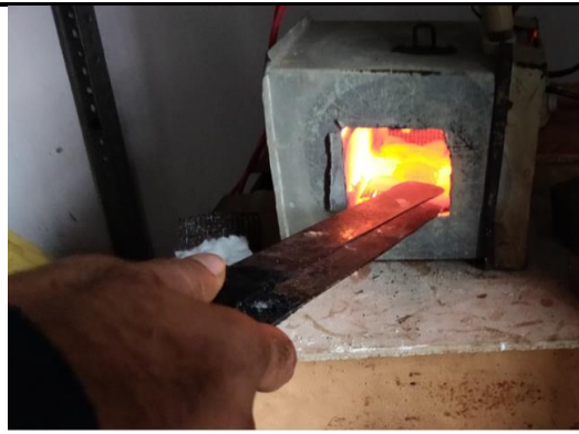
Fig.10: Handmade furnace at artisan workshop to fire meenakari products
