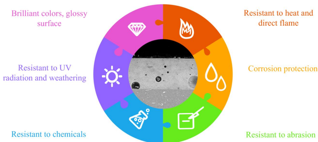
Fig. 1: Graphic representation of Vitreous enamel coating properties [6] .
