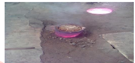
Fig 11: GRAPHITE CRUCIBLE WITH CHARGE PARTICLE
