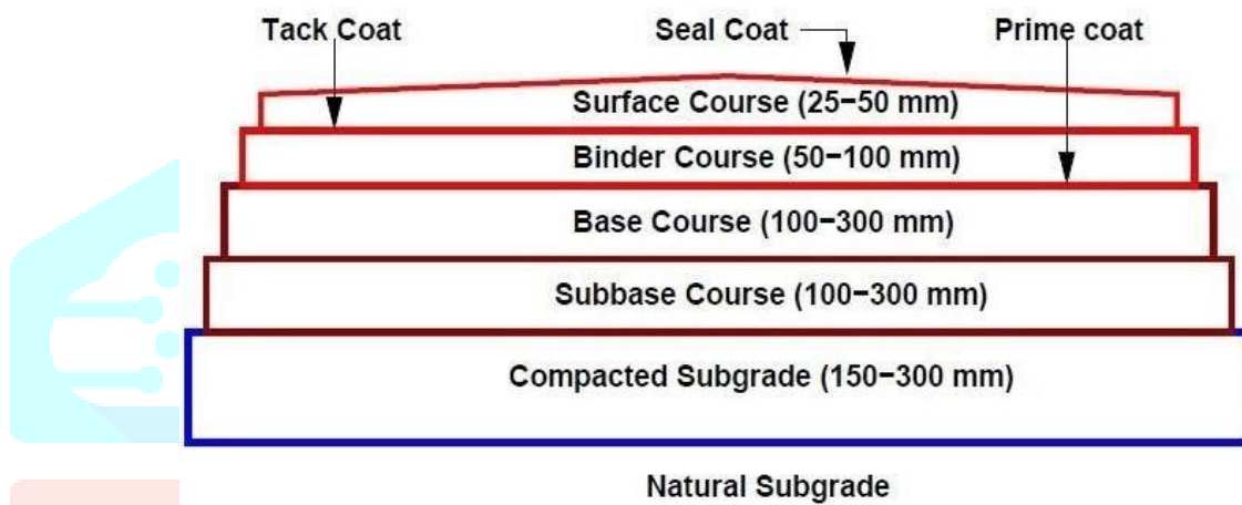
Typical cross section of a flexible pavement
