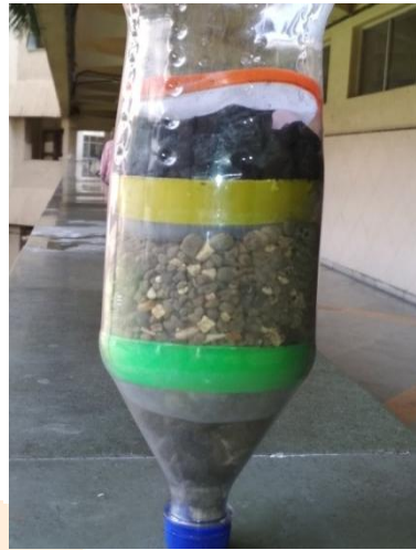
Figure 6: Sand filter with activated carbon
