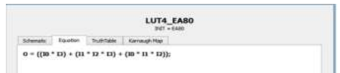
Figure 6: LUT Equation of full adder.
