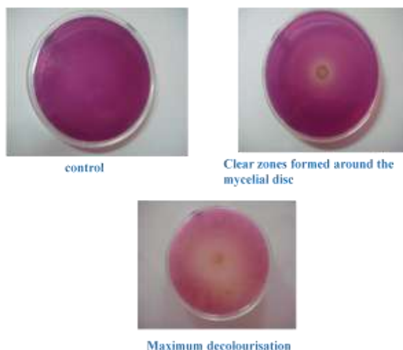
Figure 1: Screening for Decolorization of the dye RBV at 200 ppm by S. ostrea on solid media
