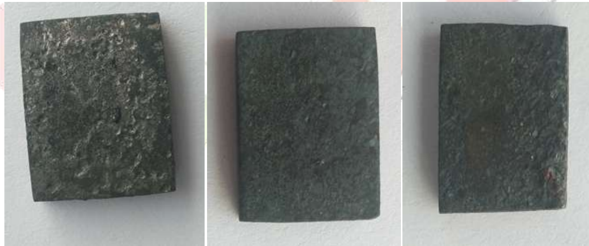
Fig. 2 Surface micrograph for the SS316L steel exposed to molten salt Na 2 SO 4 -60% V 2 O 5 at 900°C for 50 cycles (a) uncoated, (b) TiAlN coated, (c) AlCrN coated.
