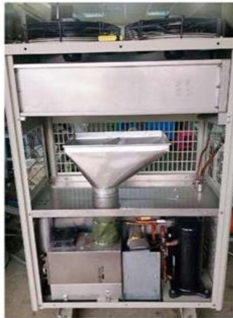
Fig.2 Supersonic vaporization chiller system
