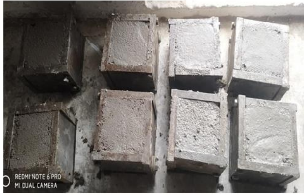
Figure 1: Casting of cement mortar cubes
